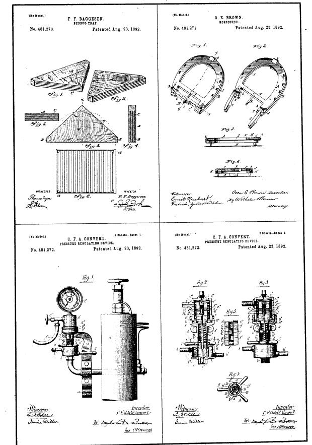
trap consisting of a block of wood triangular, or approximately so, in shape, sawed across the grain and having parallel saw-kerfs therein extending in the same direction, the corners of said block being left uncut.
